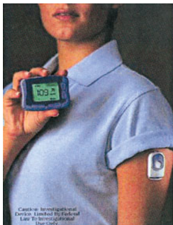
Figure 5. The investigational subcutaneously implanted continuous blood glucose monitor of Therasense, based on the electrical wiring of the enzyme glucose oxidase. From Ben Feldman, Therasense (now Abbott Diabetes Care) Diabetes Technology Meeting, November 6-8, 2003, San Francisco, CA.
